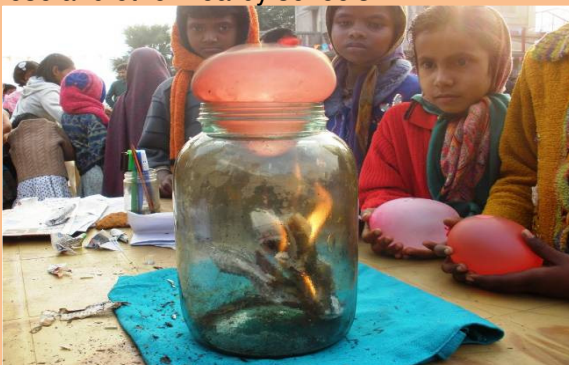
Demonstrating that air has pressure from all directions
